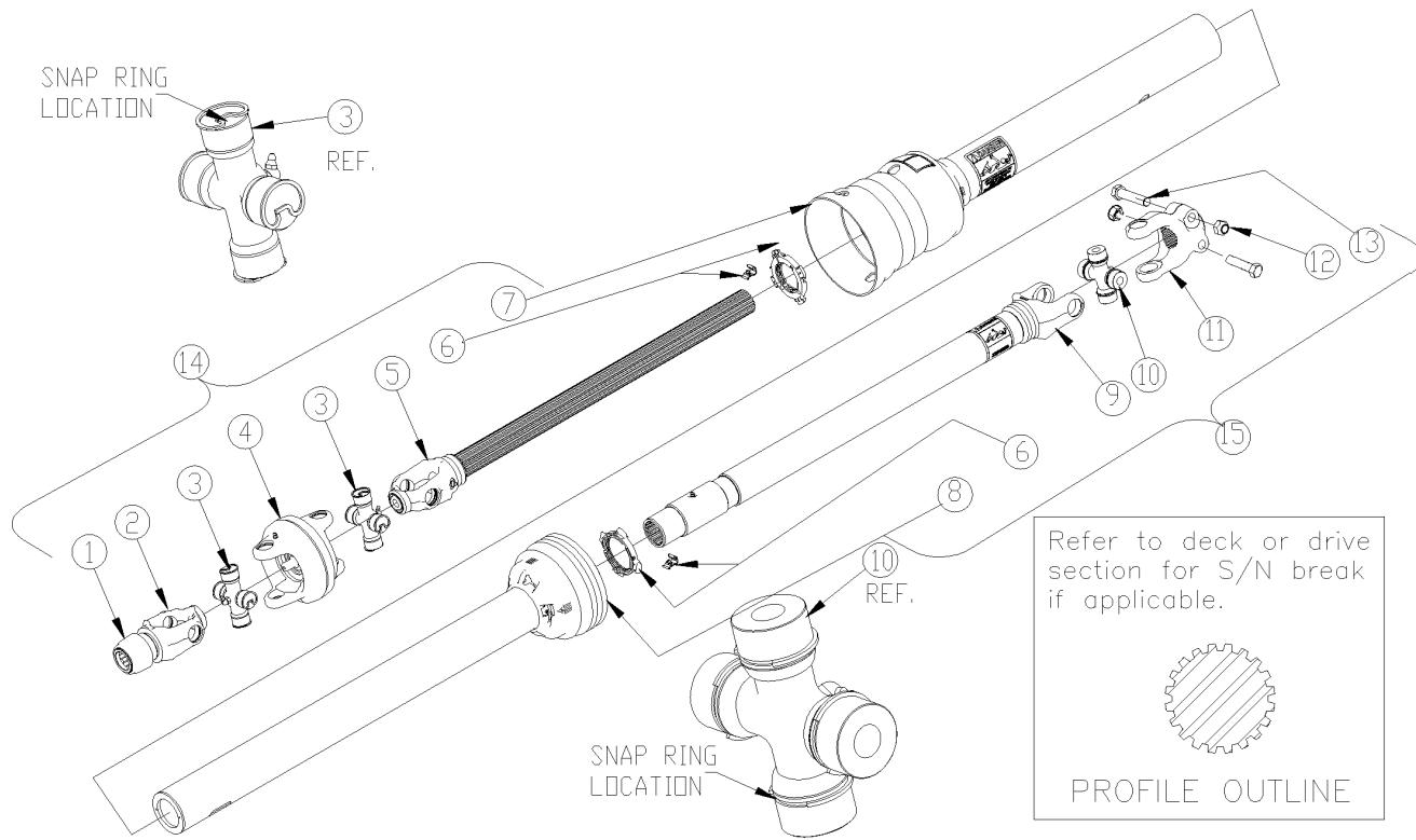
***Driveline CV 1.75 1000 RPM (826-645C)*****Applies to RCM5020 SERIES 2 S/N 1316082+**
