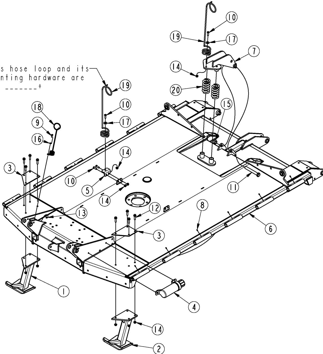
**Deck Center Components****Applies to RC5020 SERIES 2 S/N 1316082+, RCM5020 SERIES 2 S/N 1316082+**
