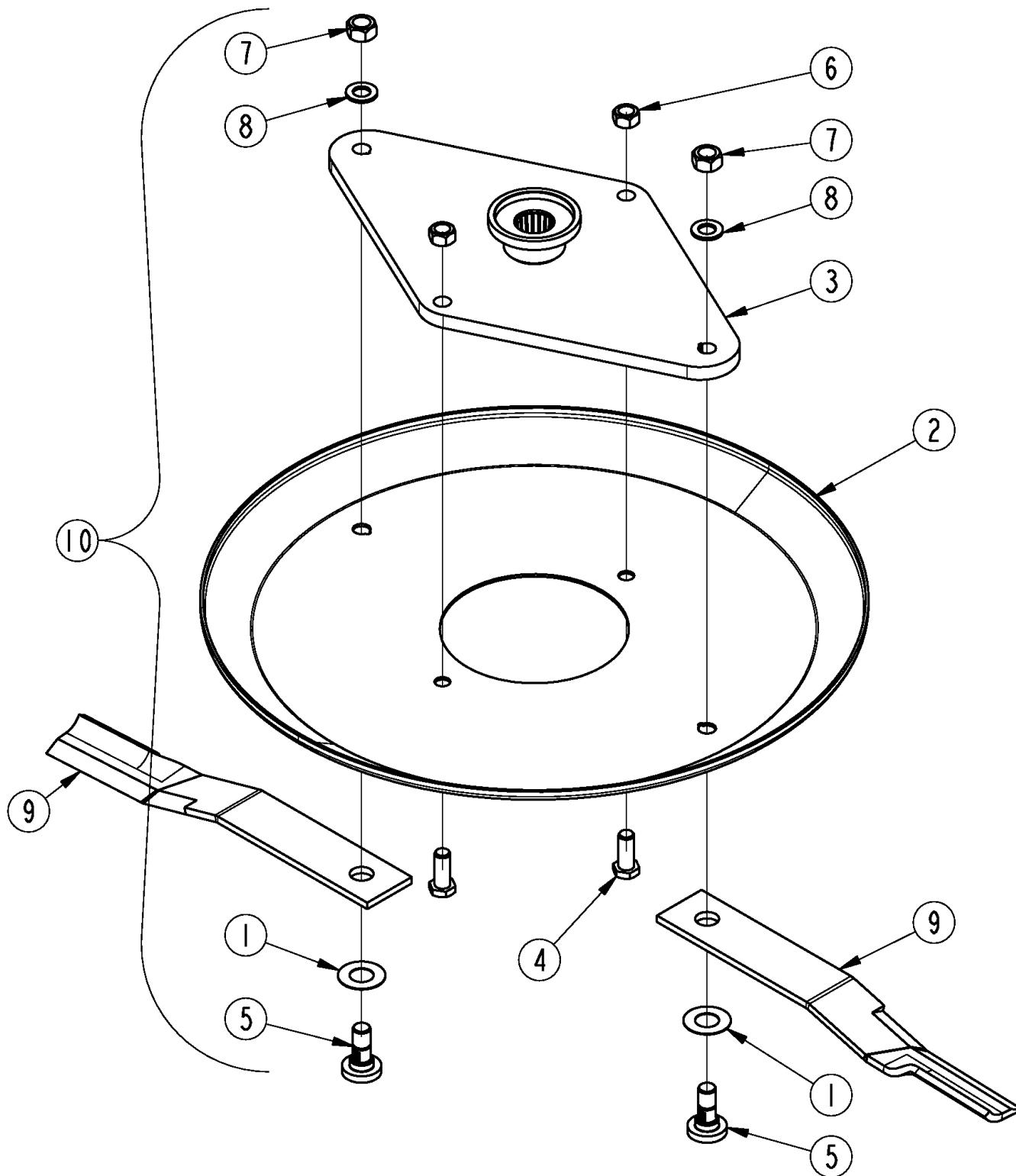
***Blade Carrier Components*****Applies to RC5020 SERIES 2 S/N 1316082+, RCM5020 SERIES 2 S/N 1316082+**
