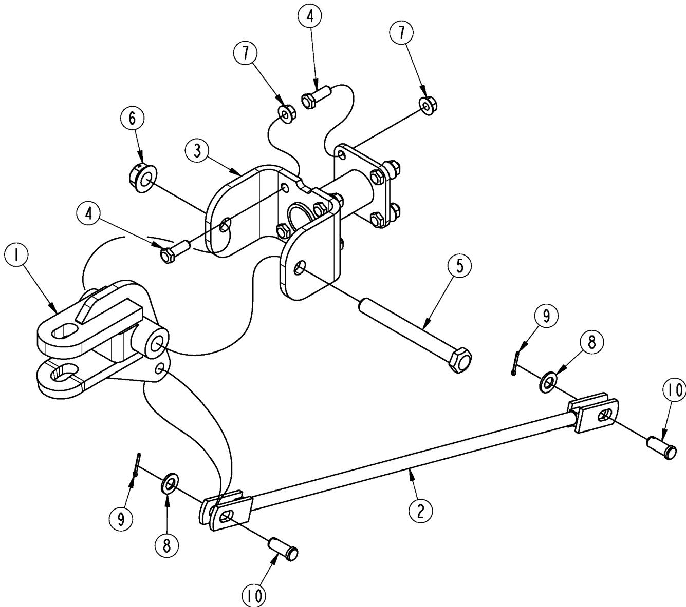
***Hitch Standard Pivoting Clevis (330-225A)***
