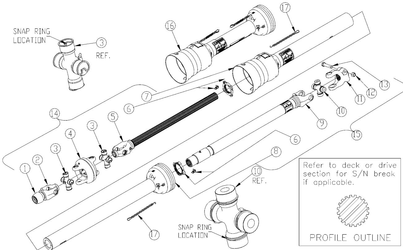
***Driveline CV 1.38 1000 RPM (826-644C) Weasler*****Applies to RCM5020 SERIES 2 S/N 1316082+**
