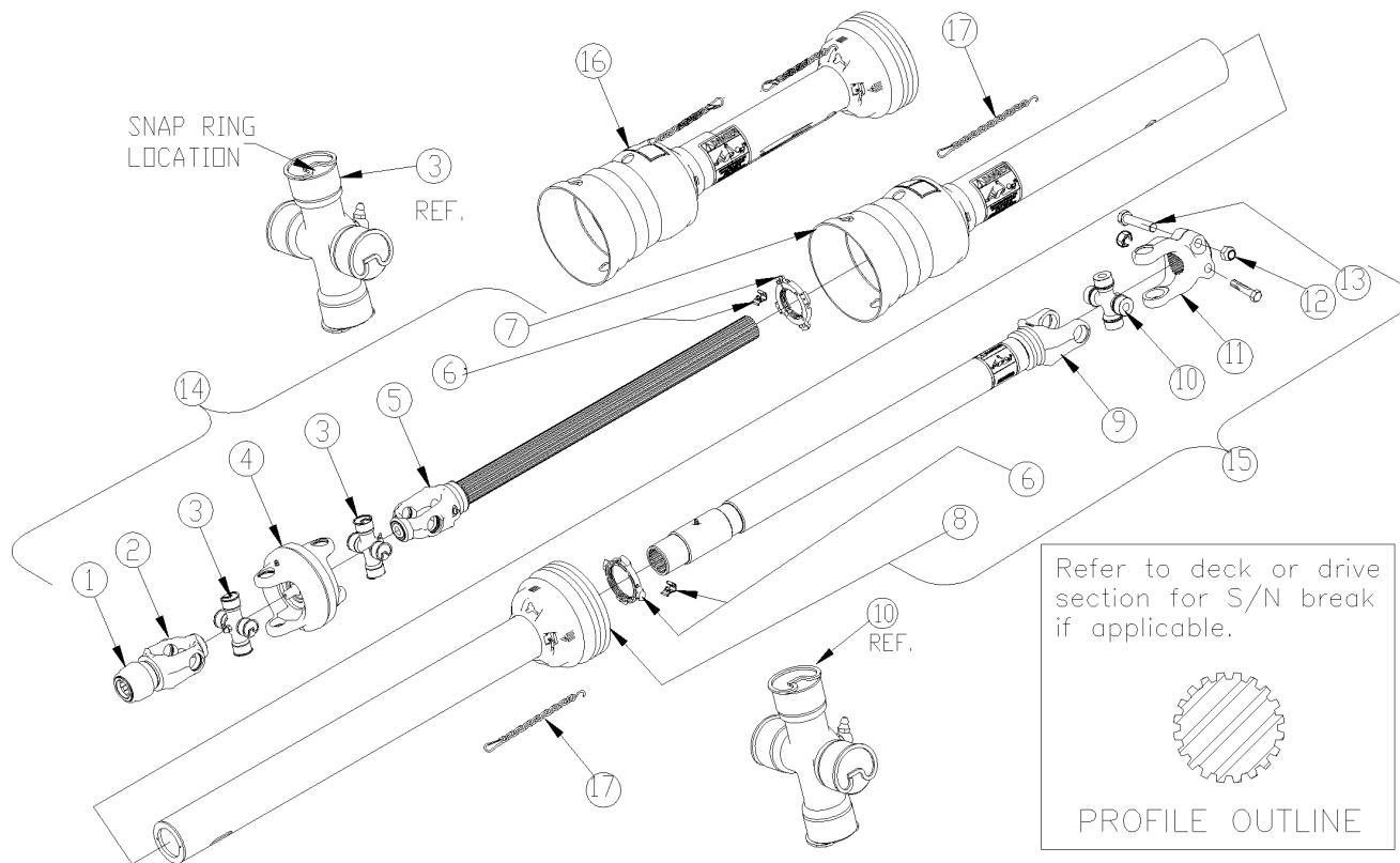
***Driveline CV 1.38 540 RPM (826-643C) Weasler*****Applies to RC5020 SERIES 2 S/N 1316082+**
