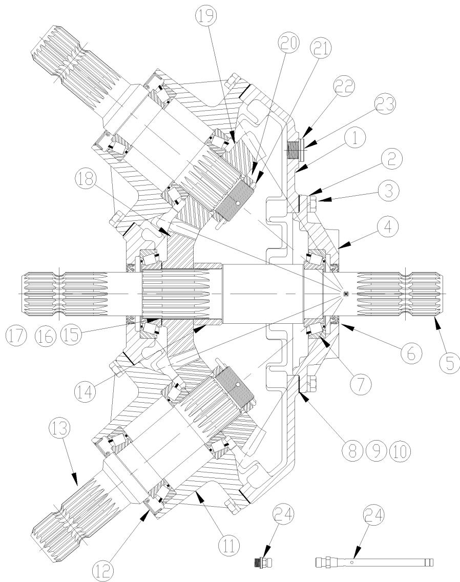
**Gearbox Divider 540 RPM (826-520C) ITG**
