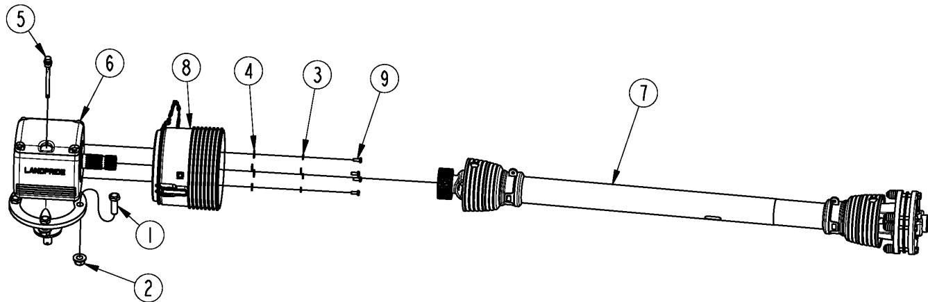
***Deck Wing Drive Components*****Applies to RC3715, RCG3715, RCGM3715, RCM3715**
