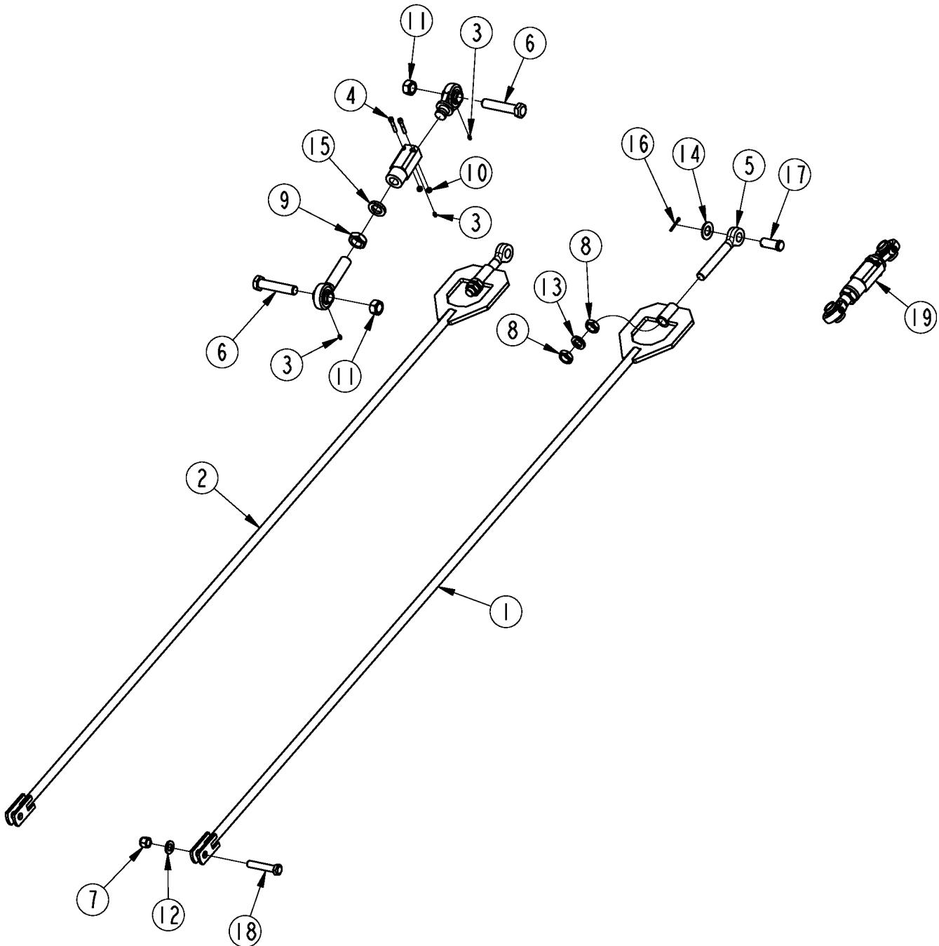
***Leveling Rods & Wing Turnbuckles*****Applies to RC3715, RCG3715, RCGM3715, RCM3715**
