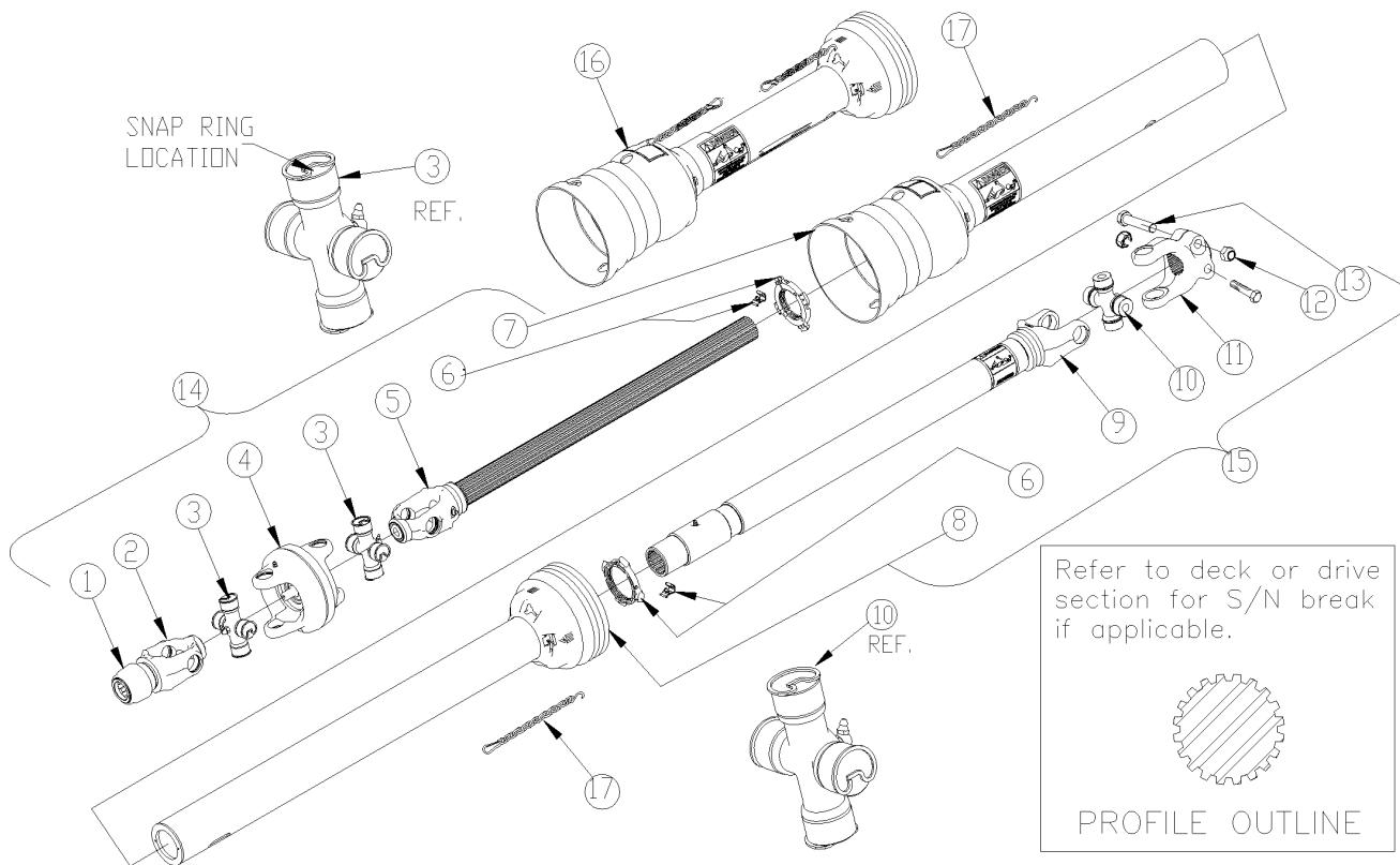
***Driveline CV 1.38 540 RPM (826-643C) Weasler*****Applies to RC3715, RCG3715**
