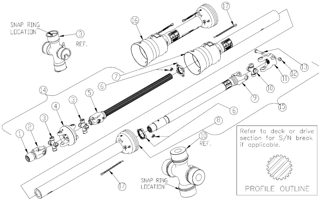
***Driveline CV 1.38 1000 RPM (826-644C) Weasler*****Applies to RCGM3715, RCM3715**
