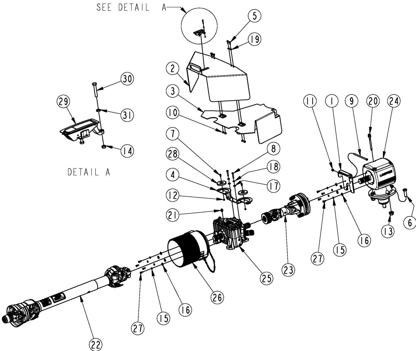
**Deck Center Drive Components****Applies to RC3715, RCG3715, RCGM3715, RCM3715**
