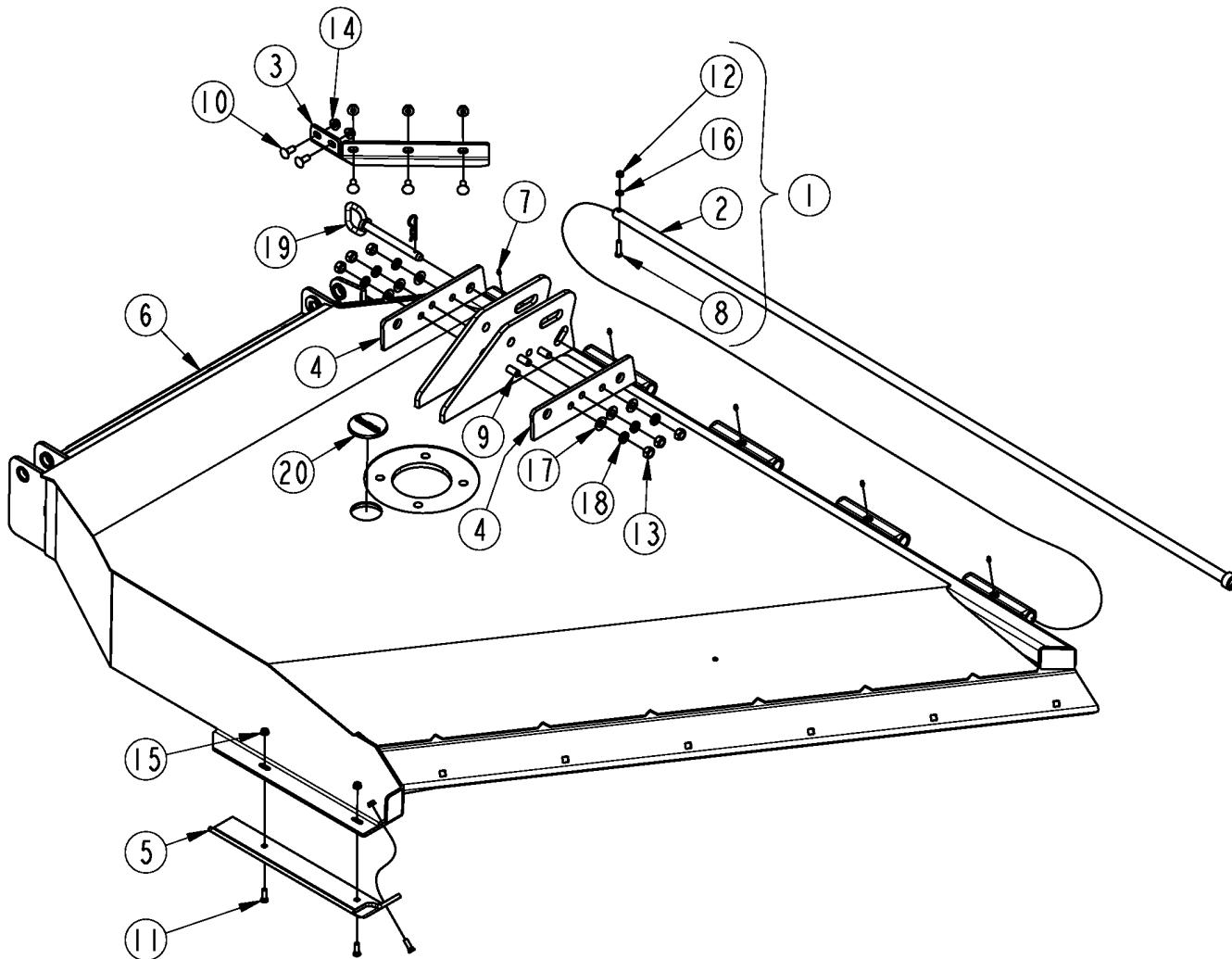
**Deck Wing Components****Applies to RC3715, RCG3715, RCGM3715, RCM3715**
