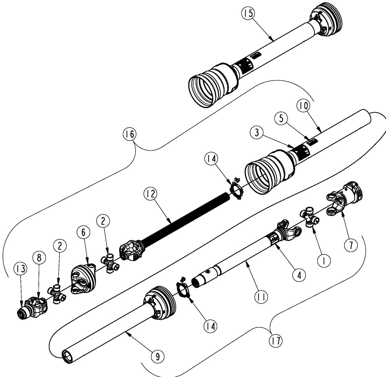
***Driveline CV 1.38 1000 RPM W/ Overrunning Clutch (826-793C) Weasler*****Applies to RCGM3715, RCM3715**
