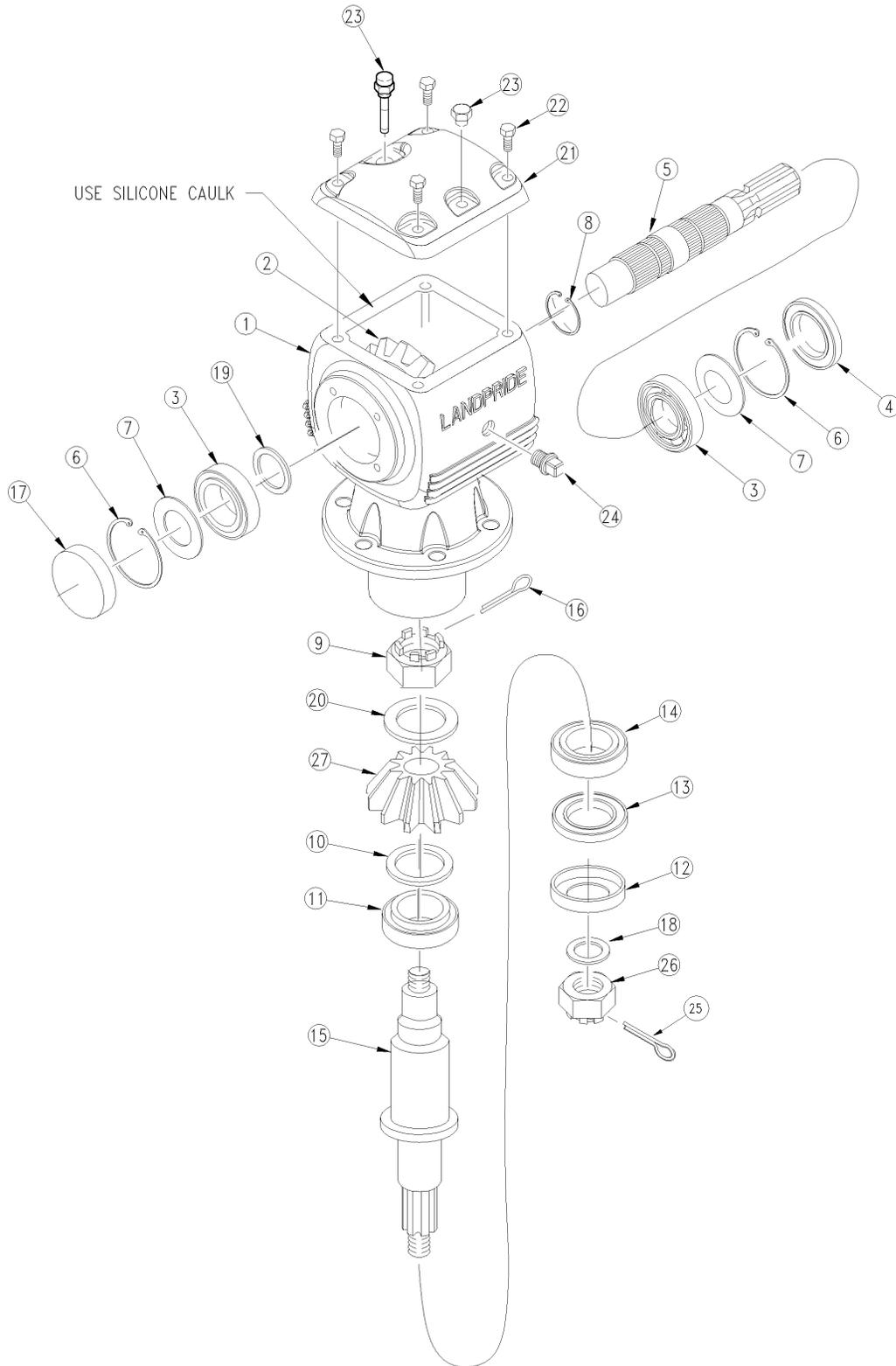
**Gearbox 540 RPM (826-316C)****Applies to RC4620**
