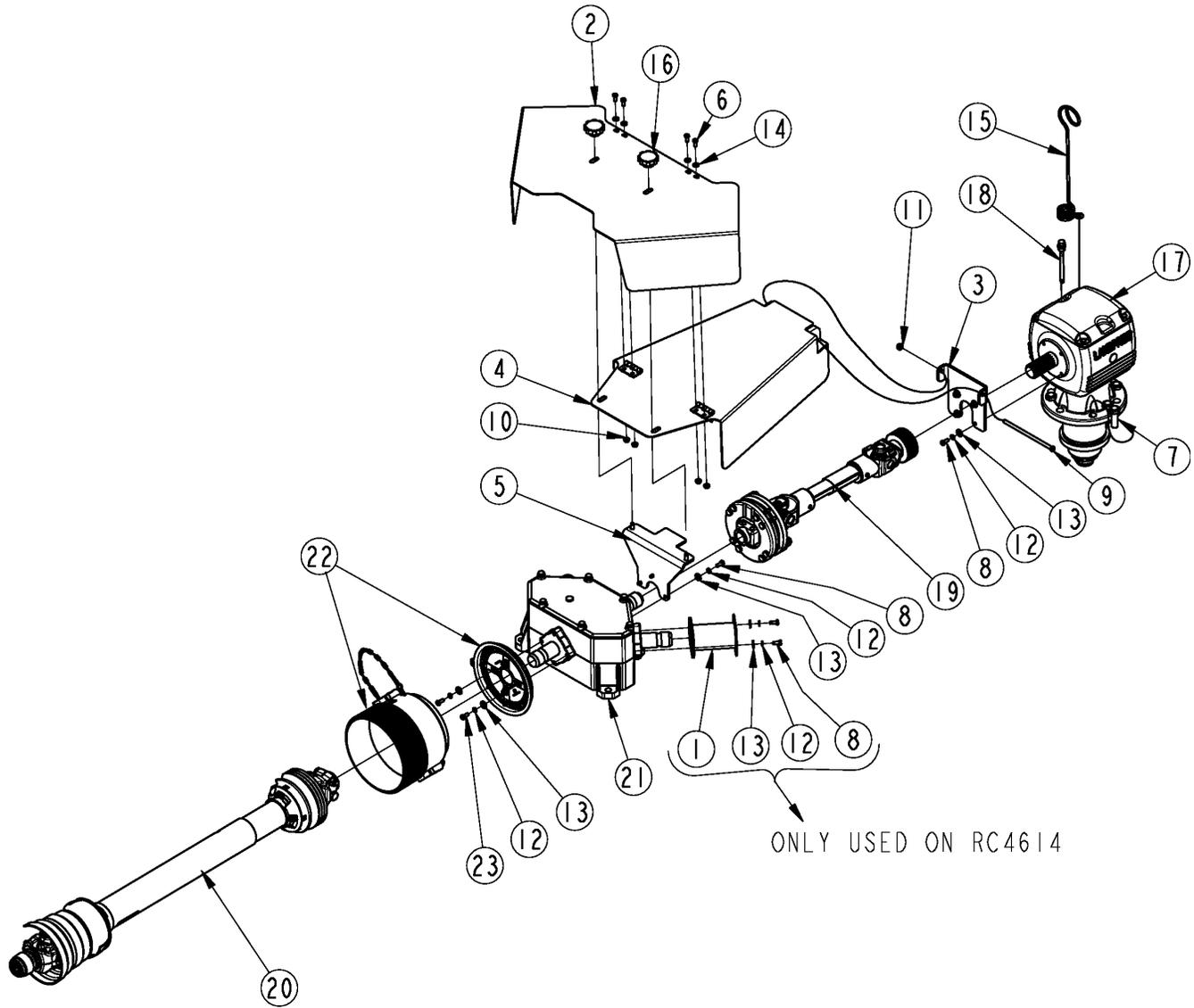
**Deck Center Drive Components****Applies to RC4620, RCM4620**
