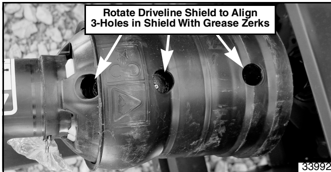
Lubrication Through Three Holes In Driveline Shield Figure 5-14
