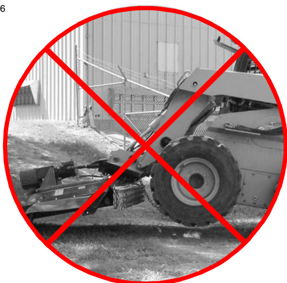
DO NOT OPERATE WITH SKID STEER FRONT WHEELS OFF THE GROUND
