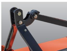
Floating 3-Point allows for easy hook-up and permits deck to follow the terrain.
