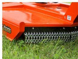
Protect against flying debris with rubber or chain guards on the front and metal band on the rear.
