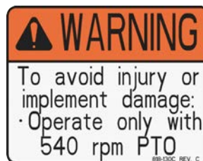
818-130C Warning: Use with 540 rpm only (RC5014)
