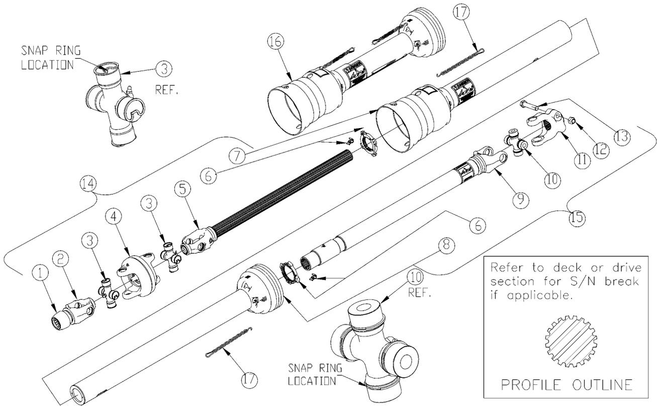
**Driveline CV 1.38 1000 RPM (826-644C) Weasler****Applies to RCM3620**
