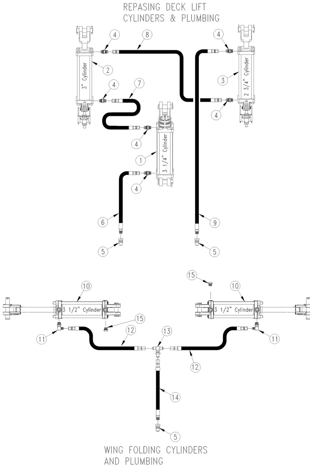
***Hydraulic Cylinder Plumbing Components*****Applies to RC3620, RCM3620**
