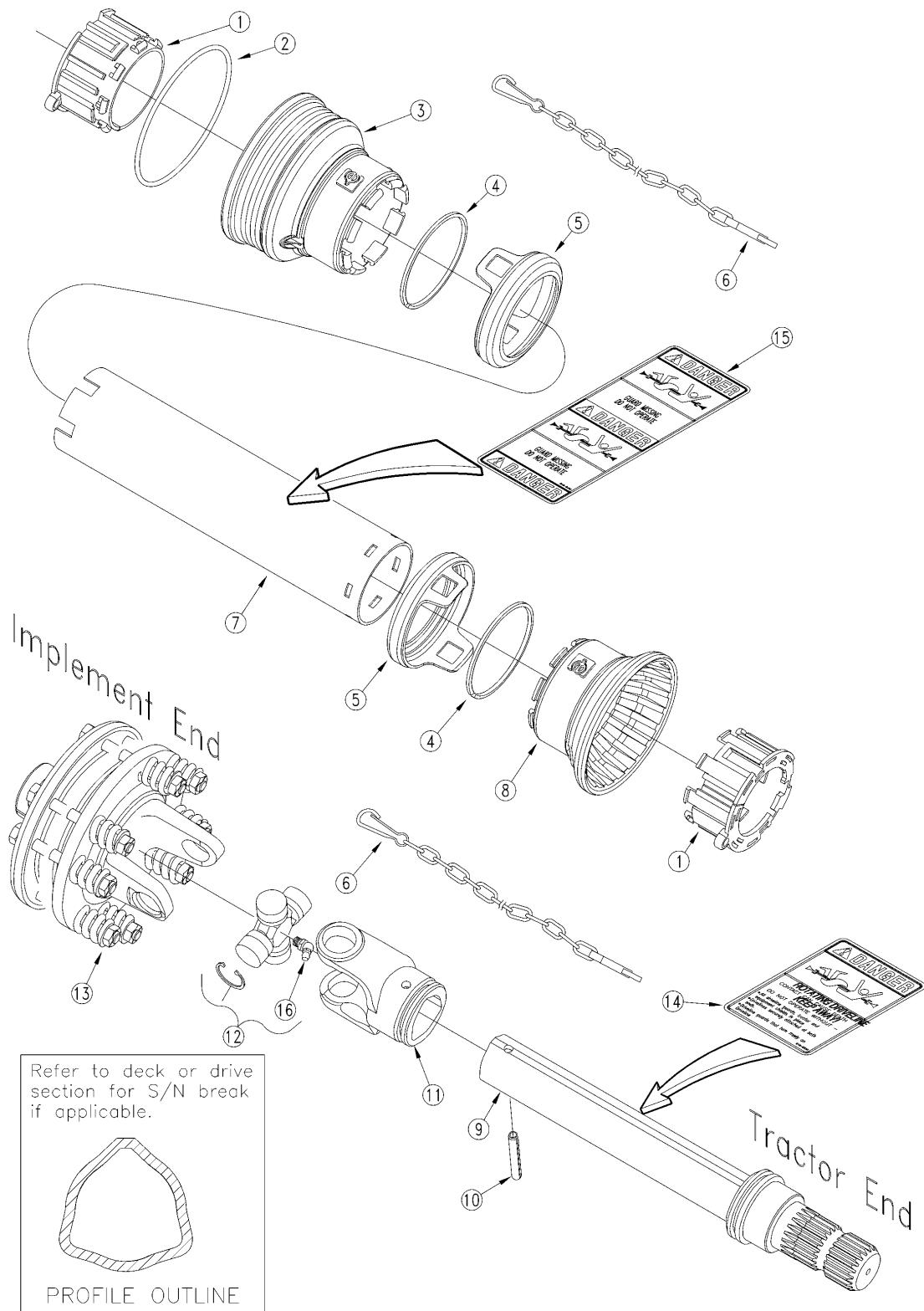
***Driveline Stub Shaft Pull Type 540 RPM (826-225C) Eurocardan*****Applies to RCF3696**
