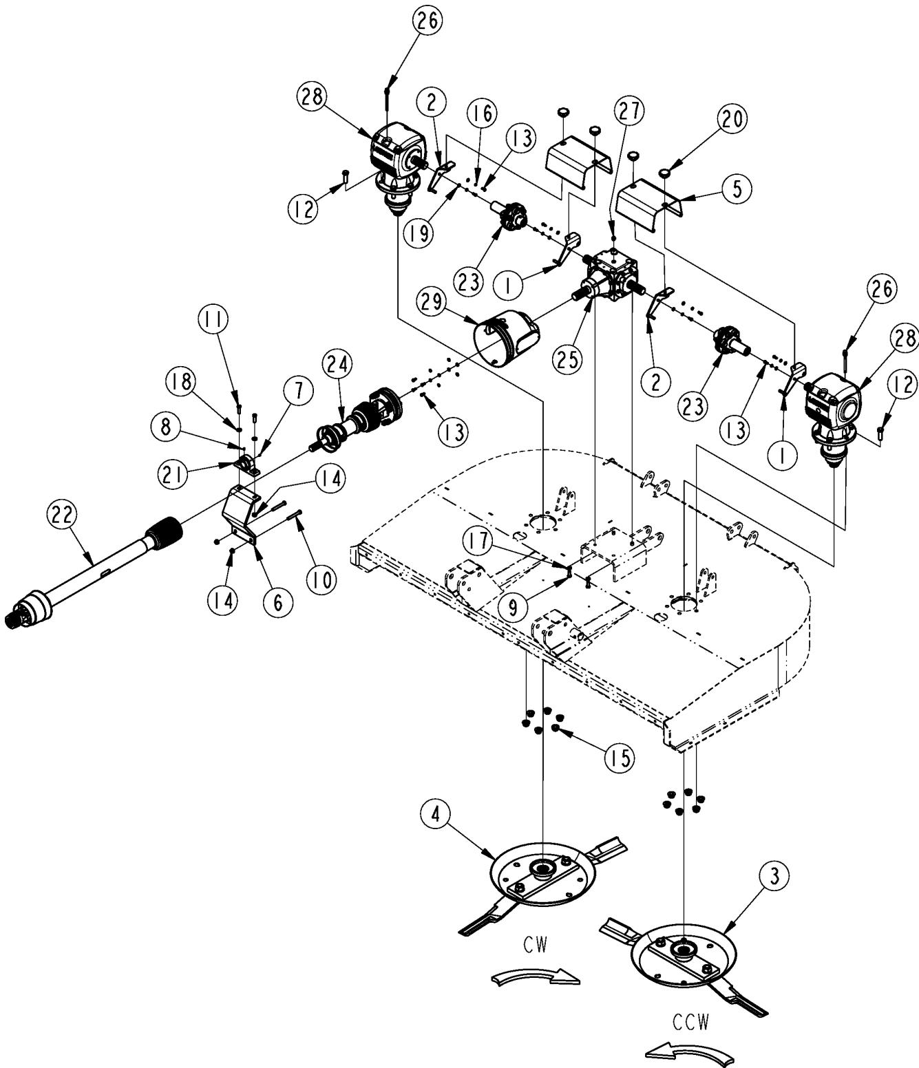
***Blade Drive Pull Type W/ CV*****Applies to RCFM3696**
