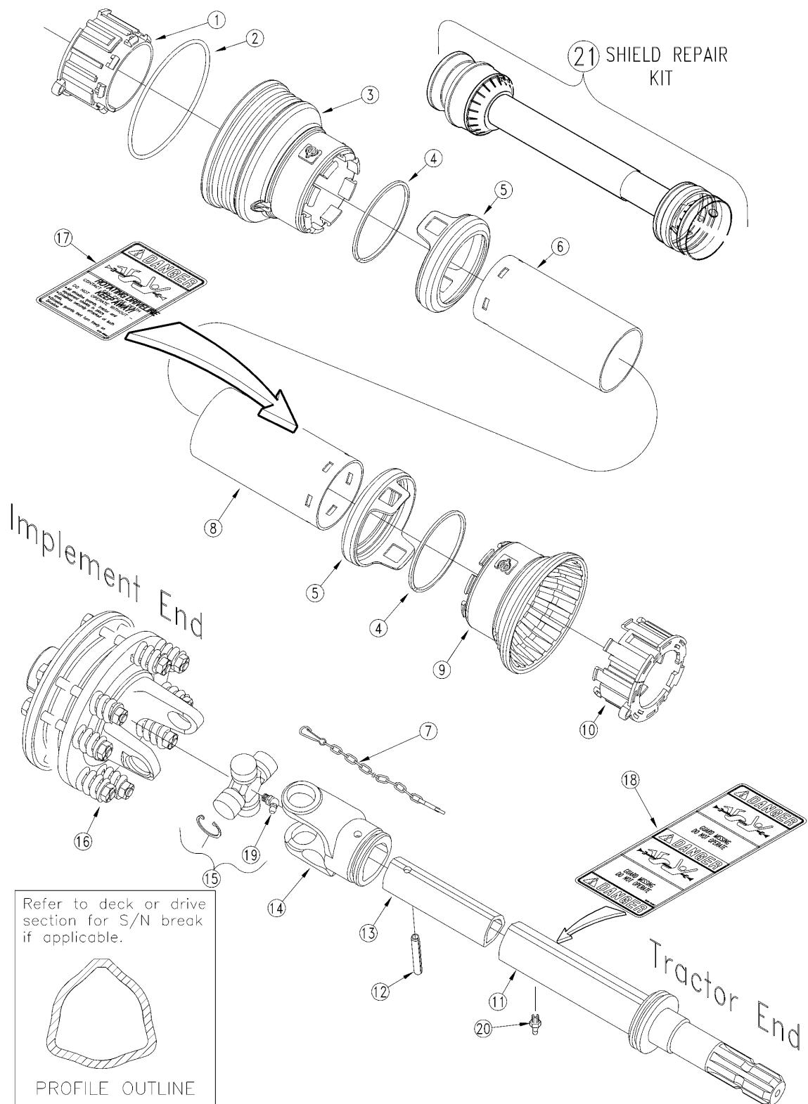
***Driveline Jackshaft (540 RPM) (826-256C) Eurcardan*****Applies to RCF3696**
