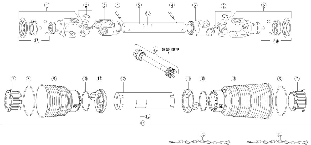
***Driveline Pull Type Conv. 1000 RPM (826-223C) Eurocardan*****Applies to RCFM3696**
