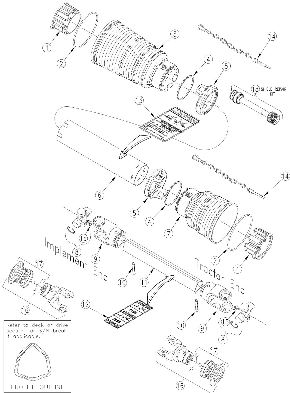
***Driveline Conv. Fixed Shaft Pull Type 540 RPM (826-151C) Eurocardan*****Applies to RCF3696**
