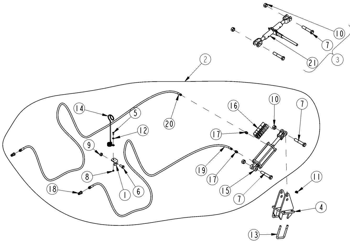
**Axle Lift Hydraulic or Manual 3-Point****Applies to RCF3696, RCFM3696**
