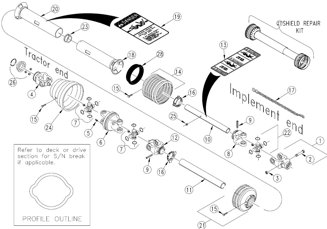
***Driveline CV Pull Type Cutter 1000 RPM (826-063C) Walterscheid*****Applies to RCFM3696**
