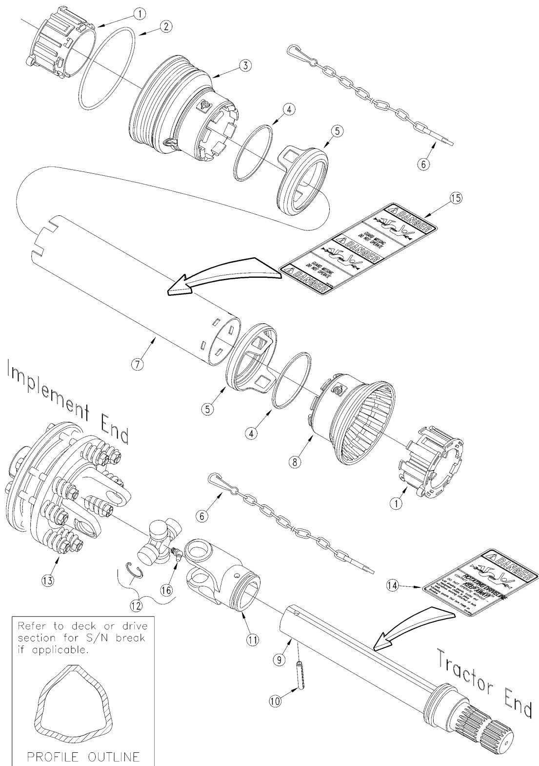
***Driveline Stub Shaft Pull Type 1000 RPM (826-226C) Eurocardan*****Applies to RCFM3696**
