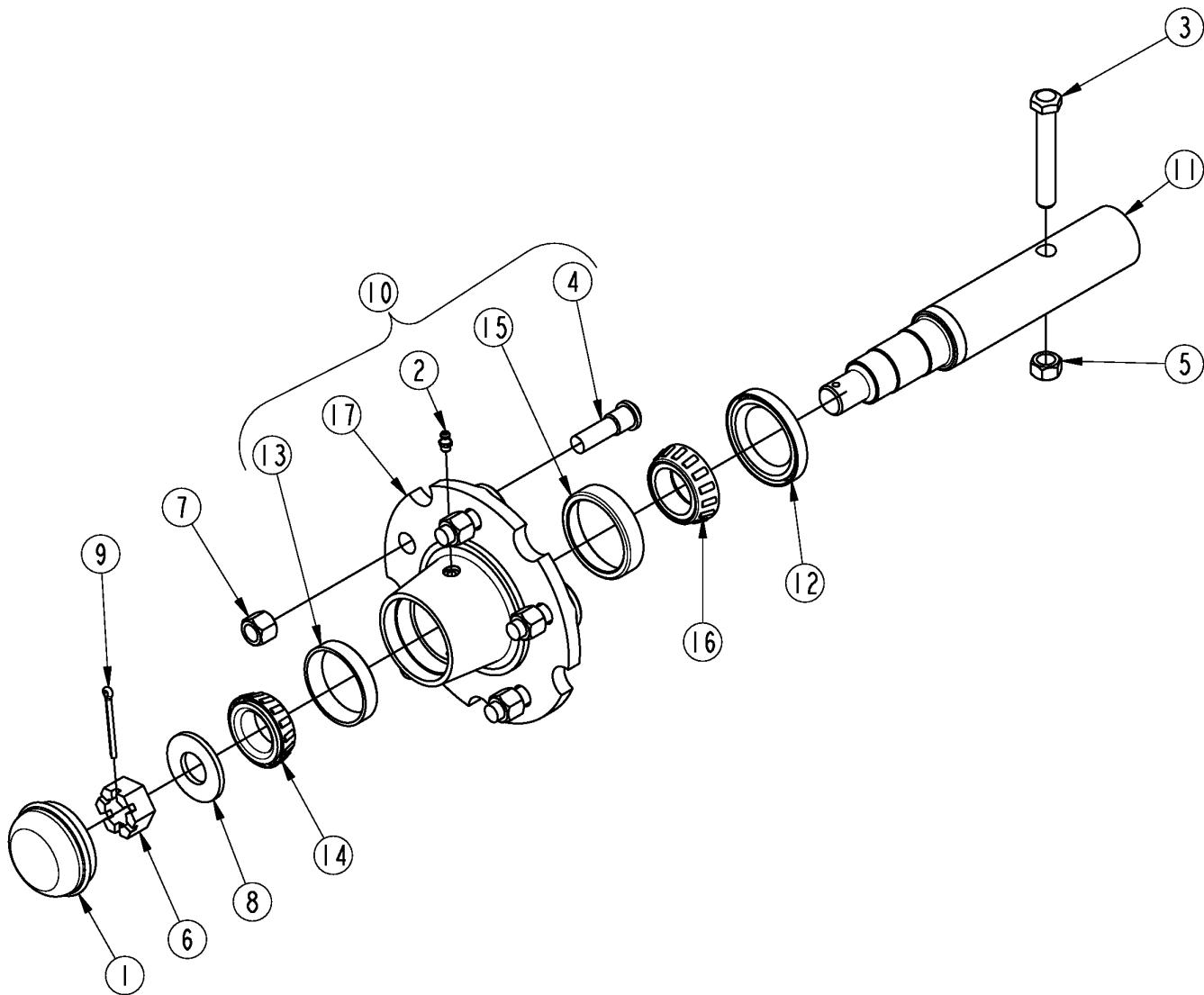
***Hub & Spindle Assembly (331-795L)*****Applies to RCF3696, RCFM3696**
