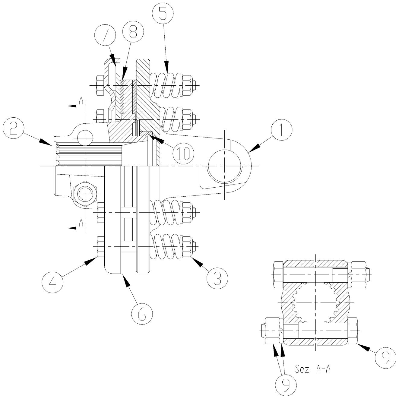
***Driveline Slip Clutch (1406128) EC*****Applies to RCFM3696**
