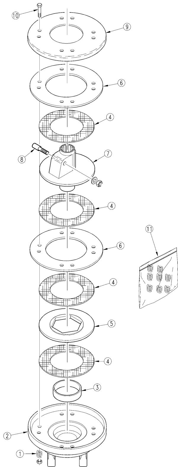
***Driveline Slip Clutch 540/1000 RPM (1446016) EC*****Applies to RCF3696**
