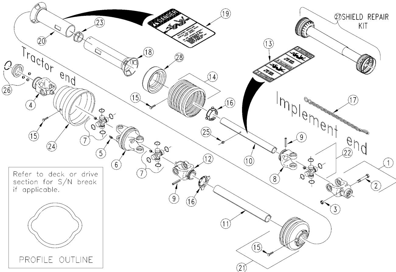
***Driveline CV Pull Type Cutter 540 RPM (826-053C) Walterscheid*****Applies to RCF3696**
