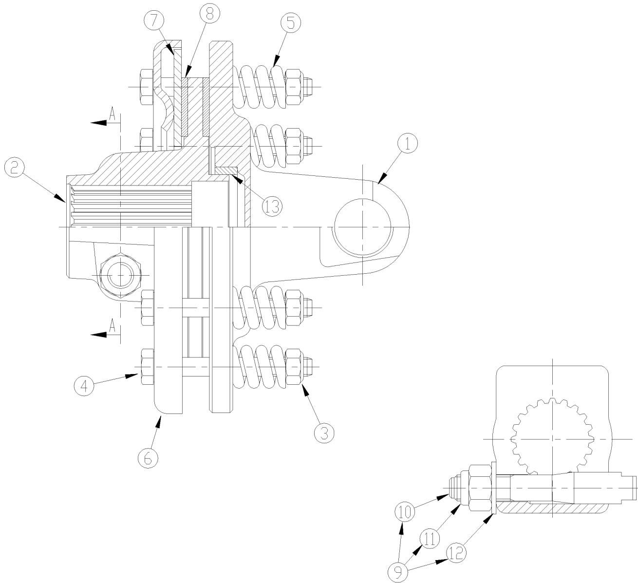
***Driveline Slip Clutch 1000 RPM (1406116) Eurocardan*****Applies to RCFM3696**
