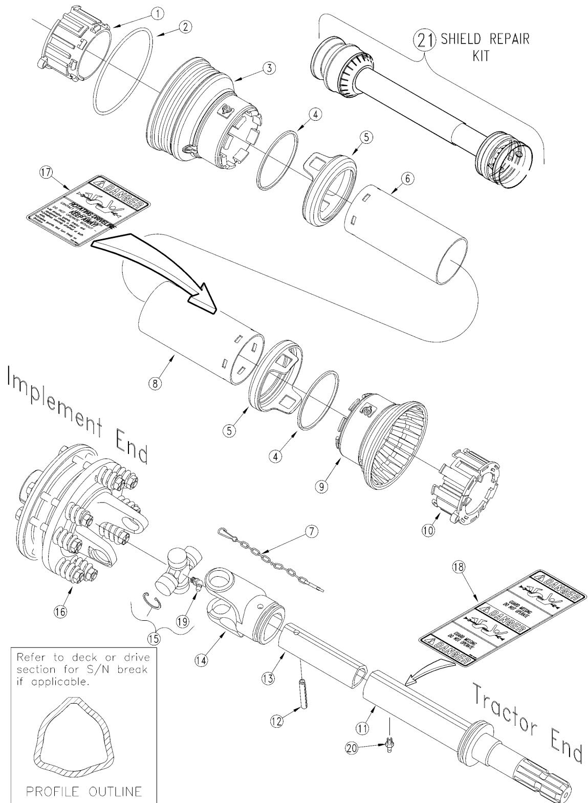
***Driveline Jackshaft (826-152C) EC New Shielding*****Applies to RCF2784**
