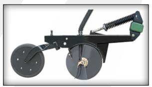
Great Plains 00 Series Openers are designed for min-till fluted feed drills. The 00 Opener features 13.5" (34cm), 4mm blades mounted on 205 triple-lip sealed bearings. The 00 Opener has a 1/4" (19mm) lead opener blade. A rear depth-controlling press wheel uses a T-handle adjuster to provide 18 depth settings.
