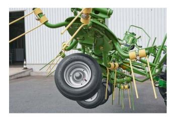
Tedding at a steep angle, turning at a shallow angle Setting the angle from 13 to 19 degrees is an easy job, which is carried out quickly on a pin-and-hole system on the brackets that hold the wheel arms. The steep position is preferred during tedding; the shallow position is best for turning. Also, the angle setting system adapts the rotors accurately to the stubble height and yield, ensuring thorough work across the full work width.
