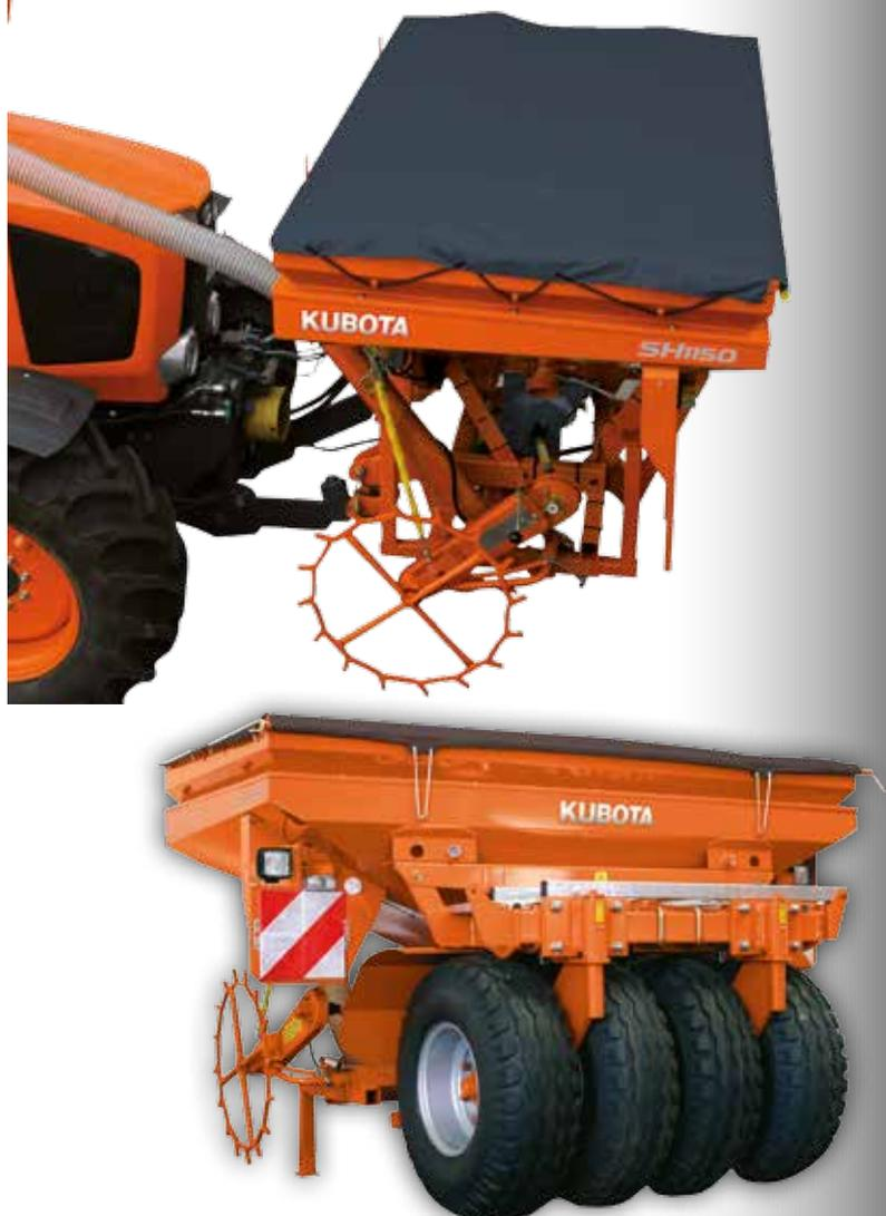
The modular structure of the Kubota SH1150 ensures even weight distribution across the machine arrangement, giving the tractor maximum balance. This improves both safety and manoeuvrability, whilst at the same time giving the driver an unrestricted view over the entire machine set-up.
