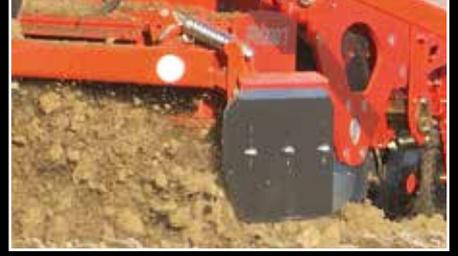
Floating side deflectors with overload protection allow smooth operation and a ridge free soil surface.
