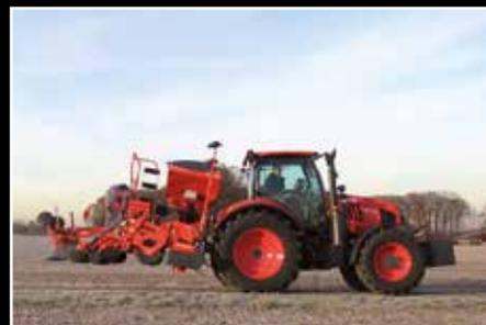
*The heavy modules (hopper and power harrow) are positioned directly behind the tractor. This arrangement optimises the position of the centre of gravity, meaning less lifting power is required, and ensures the manoeuvrability of the tractor. Road lights are fitted as standard, ensuring safe road transport at any time of the day or night.*
