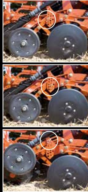
The CX-disc coulters ensure exact seed placement under both wet and dry conditions. Due to the combination of convex steel disc and flexible plastic disc, there is no need for independent scrapers saving the costs for expensive wearing parts.
