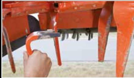
Quick-Fit tines – the tines are locked in position by a pin and clip. Tines are quickly replaced without tools.
