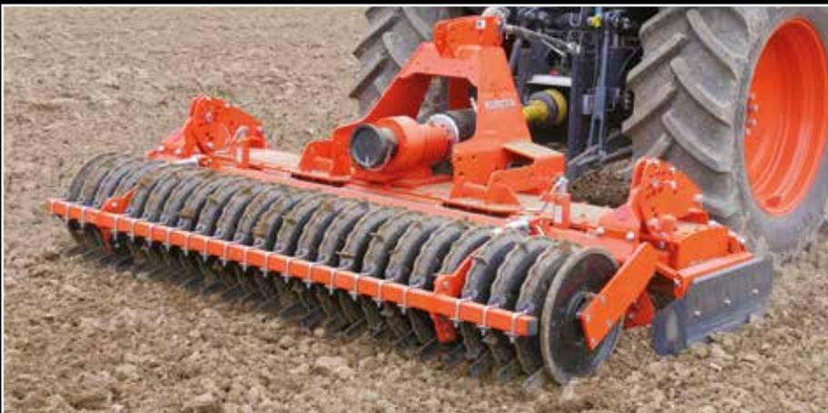
Helical (spiralled) tine positioning reduces peak loads on the driveline, resulting in smoother running. The tines are arranged at different angles in order to ensure even levelling and help prevent damage by stones. Savings are also made in terms of fuel consumption.
