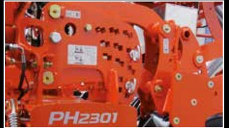
The depth adjustment is positioned closer to the headstock to reduce stress on the whole construction and to allow the ease of fitment of all Kubota packer roller types.
