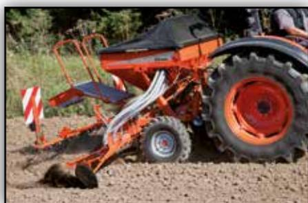
*Compact construction for minimum lifting requirement*
