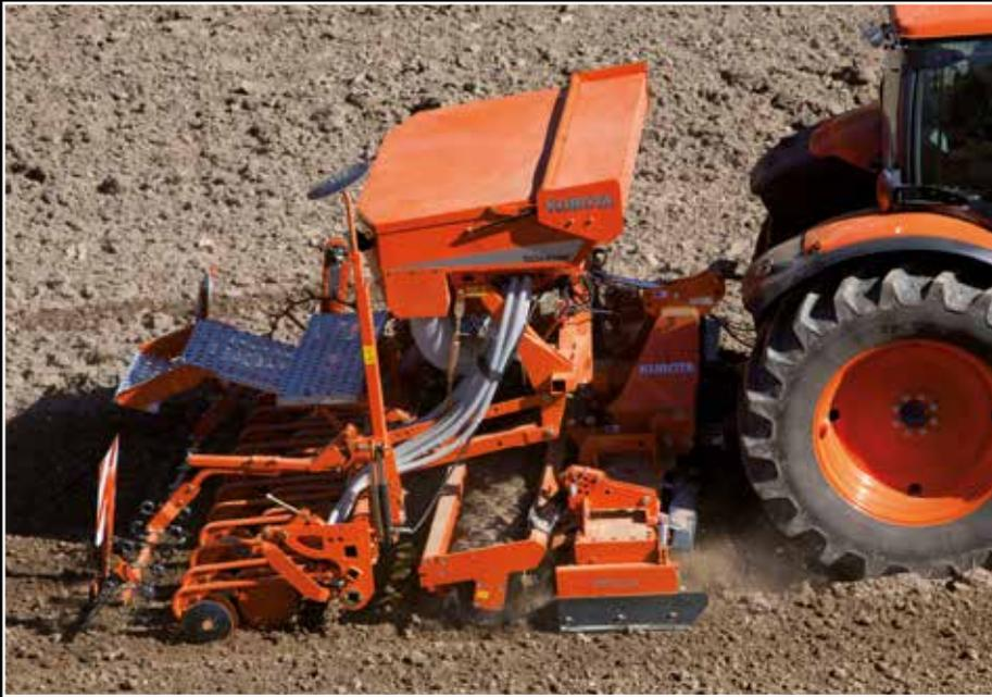
The Kubota SD2000M Series is the heavyduty version of the SD1000M. Available in working widths of 3.00, 3.50 and 4.00m it is a highperformance machine for large farms and estates.
