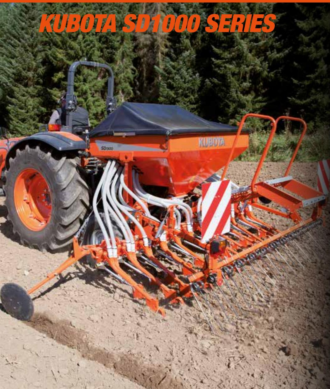
The SD1000 Series is the ideal machine for small and medium-sized farms and combines a compact, light design with the proven Kubota quality. Working widths from 3.0 to 4.5m are available. The power requirement is from as little as 55 kW due to the close centre of gravity.
