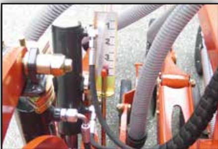
The sowing depth can be adjusted toolless by spacers which are located at the two outer hydraulic cylinders. The operator can see the coulters pressure setting on the scale which is easily visible from the tractor cab.
