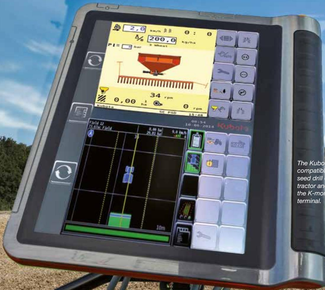
The Kubota M7001 series are ISOBUS 11783 compatible. This means that the pneumatic seed drill can be plugged directly into the tractor and where available be operated via the K-monitor without any other separate terminal.
