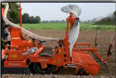
Kubota PH3300 with coulters CB1300 in combination with the front hopper SH1150.
