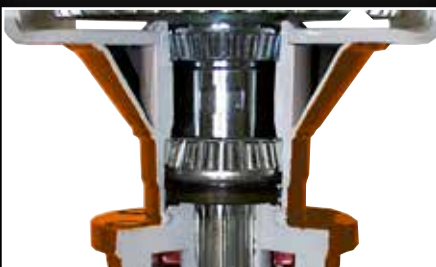
Two large conical bearings with a wide distance provide rigidity and a long service life.
