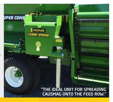
The hydraulics plumb into the main hydraulic supply and has a flow adjuster to regulate the feed rate.
