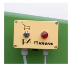
The swath boards turn to the left or right, the drawbar swings in or out into work or transport position. The operator selects the individual functions on the electric control box.
