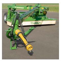
Useful – the stand folds down for sure footing. The pto shaft and all oil lines are stored in convenient holders. The two-point headstock moves to the side for easier attachment to the tractor.
