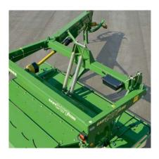
Adjust the ground pressure conveniently to requirements. Adjustable coil springs provide quick and optimum adaptation to all conditions. The system stands out for its large choice of setting options and convenient handling.
