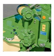
Cutterbar and conditioner share the same gearbox, which also integrates the two-speed mechanical CV conditioner gearbox (600 rpm and 900 rpm).
