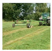
The EasyCut 3210 CV, 3210 CRi and 4013 CV models feature a mid-mounted drawbar with hydraulic control to swing to the right or left of the tractor. These are the ideal machines for cutting large fields.
