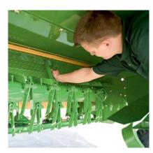
The EasyCut 2801 CV, 3200 CV, 3201 CV, 3210 CV, 3600 CV and 4013 CV models feature a wide V-steel tine conditioner, where the pivoting V-type tines provide uniform conditioning across the full work width.
