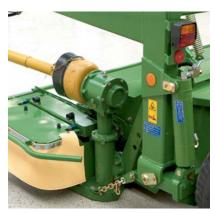
Frictional connections – drive power to the roller conditioner flows directly and slip-free via gearboxes. The gears that drive the bottom roller are integrated in the cutterbar gearbox behind the left top hat.
