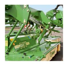
Excellent ground following – thanks to two staggered cutterbars rather than one full-width cutterbar. The two units operate independently of each other and follow every ground contour. EasyCut 6210 CV is the machine to produce quality forage.
