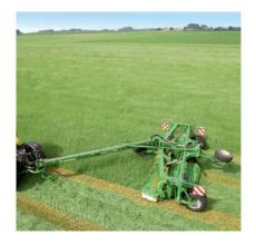
EasyCut 2800 CRi, 3200 CRi and 3210 CRi featuring conditioner rollers. The full-width and chevron-profiled rollers interlock and deliver superb treatment of legumes and other leafy crops.
