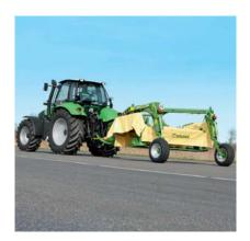
Nice and compact. Running inline behind the tractor, EasyCut 3200 does not exceed the statutory 3.00 m (9'10") transport width, gives plenty of ground clearance and is approved to 40 km/h (25 mph) maximum speed. This is the machine to travel quickly between sites.
