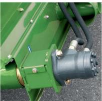
Powerful hydromotor and infinitely variable conveyor speed – the perfect match to set windrow widths to requirement for the following harvester.
