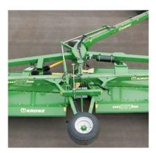
Swing left, swing right – the mid-mounted drawbar swings hydraulically to either side of the tractor. Its double acting ram is dependable even in the most difficult conditions.
