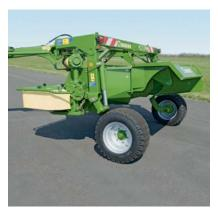
Swift – the mower lifts out and swivels hydraulically into the middle for transport on public roads, a position that gives plenty of ground clearance to run over deep ruts and windrows.
