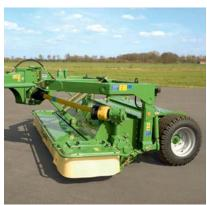
Adaptive – the mower pivots in a double frame for full up/down travel to avoid obstacles and follow ground undulations. The system's response is controlled by spring tension. The stronger the tension of the springs, the more responsive the system is.
