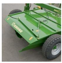
Providing infinite variable adjustment, the two swath boards are controlled by a shared linkage system and a double-acting ram that synchronizes action to the right or left.
