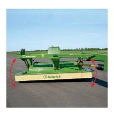
There is plenty of pivoting room on either end of the cutterbar, which allows the unit to adapt to any ground contours. As the mower pivots in its double frame, it closely follows the ground – to the effect of producing clean forage and protecting the turf.
