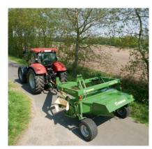
Swift 40 km/h (25 mph) road transport. Not exceeding the statutory 3.00 m (9'10") transport width, EasyCut 2800 CV/CRi, 3200 CV/CRi and 3201 CV do not require special permission to travel on public roads.
