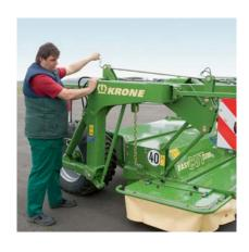
Height control is quick and convenient – thanks to crank handles that set the cutting height steplessly and separately on each unit.
