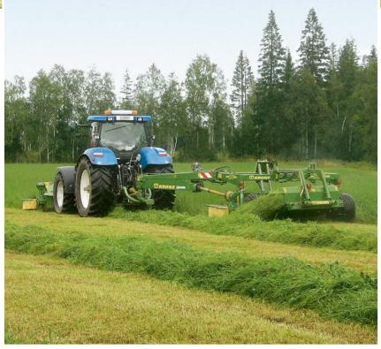
The EasyCut 32 CV and 32 CRi combination produces a double windrow in a single operation. The cross conveyor belt merger places the material onto or next to the windrow that is produced by the front mower. Eliminating the tedder and rake passes, the combination boosts your efficiency and saves your time and money. These facts suggest that gathering two windrows into one is a profitable strategy that justifies the investment of a cross conveyor belt merger.
