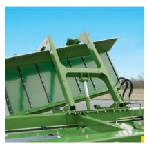
An ideal system, a single-acting ram raises the cross conveyor as a reversing valve shuts it off and back on when the ram lowers the unit back into work.
