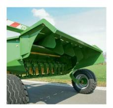
Full flexibility: The optional guide plates feature a pin/hole setting system to vary the angle. Choose between narrow windrowing in wet and boggy terrain and wide spreading, if rapid drying is the priority.
