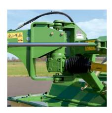
Frictional connections without belts ensure that drive power flows smoothly to the cutterbar and conditioner via gearboxes and driveshafts – thanks to two swivel gearboxes. Peace of mind comes from overload protection built into the driveline.
