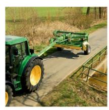
Travelling between fields at 40 km/h (25 mph). In inline position, EasyCut 3210 CV and CRi are allowed to run on public roads and at 3.00 m (9'10") transport width they do not require a special permission.
