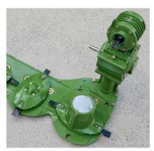
Smart by design, the cutterbar is powered by a right-angle gearbox, which is arranged right behind the inner top hat – for blockage-free operation on the headland and in awkwardly shaped fields.
