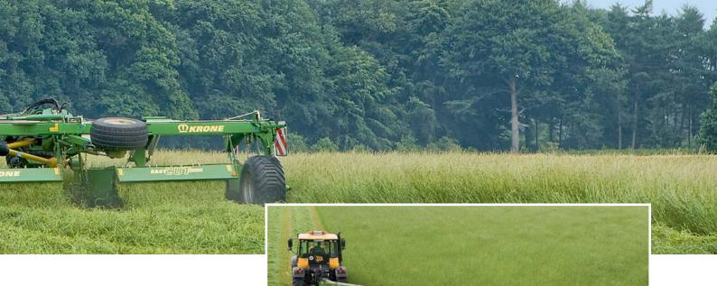
Take the choice – EasyCut 6210 CV cuts to the right or left of the tractor. Simply swing the drawbar to the other side as you do the headland turn and match up with the previous pass without mowing in beds. The tractor is not running in standing crop so that clean and loss-free cuts are guaranteed. You always use the machine to potential and, in combination with a front-mounted mower, at full width capacity. In sloping fields, it allows the tractor to run always on the hillside.
