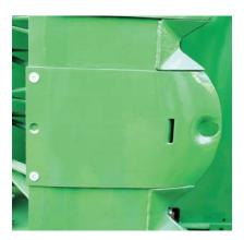
Floating over the turf, extremely wide skids made from hardened steel are bolted to the cutterbar to protect the unit and the turf. High-cutting skids are available to produce longer than 80 mm (3") stubble. Depending on the installation, these skids increase the cutting height by 30 mm (1") or 50 mm (2").
