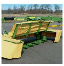
Easy to maintain: The front section of the frame folds up to give easy access to the discs for cleaning and convenient blade replacement.
