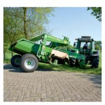
Plenty of ground clearance – single-acting rams raise the double frame and the mower for road transport and when crossing windrows. A tap locks the rams during road transport.
