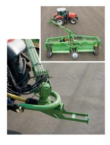
Turns on the spot – the swivel-head gearbox (1,000 rpm) on the two-point headstock provides the flexibility to turn through 90° and larger angles while the main driveshaft does not move, allowing drive power to flow vibration-free to the cutterbar.
