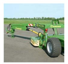
Constant pto speed – thanks to a driveline that is comprised of driveshafts and gearings, which effectively transfer the drive power to the discs, even when operating in heavy crops and at wide working widths. The main gearbox on all trailed EasyCut mowers matches a 1,000 rpm pto as standard fit.
