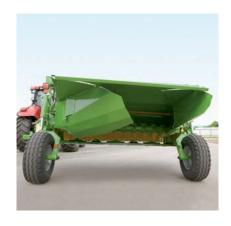
Forming perfect double windrows, the long and pivoting swath boards tighten the material flow and windrow it neatly to the side, forming fluffy double windrows for easy pick up by the harvester.
