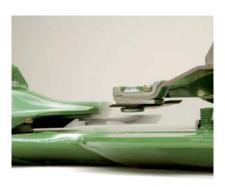
Unlimited spin - the knives are free to spin through 360°. They are hard-wearing and self-cleaning, well protected and will not interfere with the knives on the neighbouring discs.
