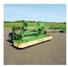
DuoGrip – parallel linkages distribute the load on the machine. Suspended in its center of gravity, the mower receives additional control by a linkage system on either side of the machine. This DuoGrip system absorbs any lateral loading on the machine, reduces the loading on the center-of-gravity suspension system and adds to the rugged design of the mower.
