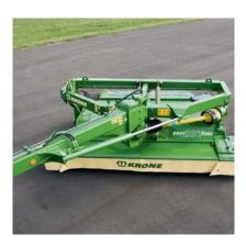
Changing sides is easy and convenient from the tractor seat. The double-acting ram swings the mower over to the other side in up and down operation and swings it centrally behind the tractor in transport position.
