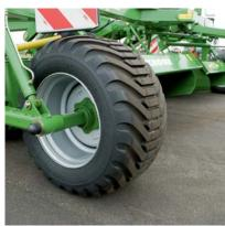
Light treading and easy pulling – the EasyCut 6210 CV models run on oversized wheels and 500/45-22.5 tires in standard configuration. These have proven best in soft terrain.
