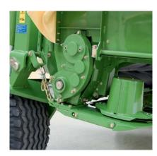
Two rollers, two gearboxes. The top roller is driven by a separate gearbox on the right end of the cutterbar and is synchronized with the bottom roller.
