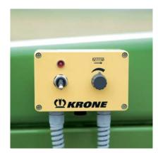
Operator comfort – the operator changes belt speed conveniently from the cab by operating a rotary potentiometer, which controls the throw and placement of the crop on top of the existing windrow or next to it.
