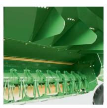
Top-quality forage – the high-capacity conditioner rotor with pivoting V-steel tines and mechanical gearbox condition the forage across the full work width and at 600 rpm or 900 rpm. Optional deflectors direct the material flow for full-width spreading and rapid drying.
