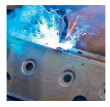
The rugged and absolutely leak-free cutterbars from KRONE are fully welded by advanced robot and CNC technologies to achieve the highest-quality build. After all, the cutterbar is the heart of a disc mower.
